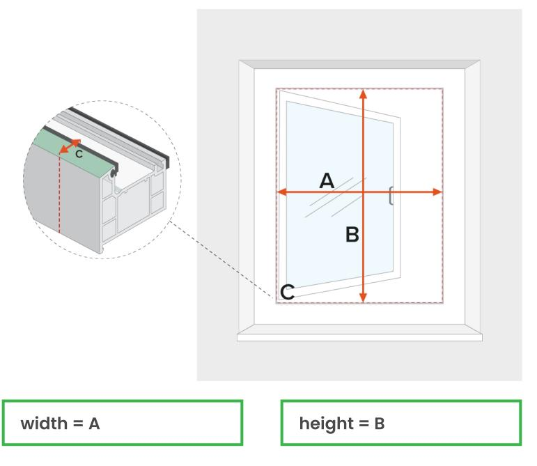
Specify the height and width of the window opening in the configurator, by measuring the edges of the window frame (reveal) from the outside.
