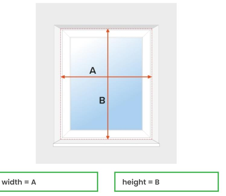
Measure the width and height of the frame (inner edges of the recess).
