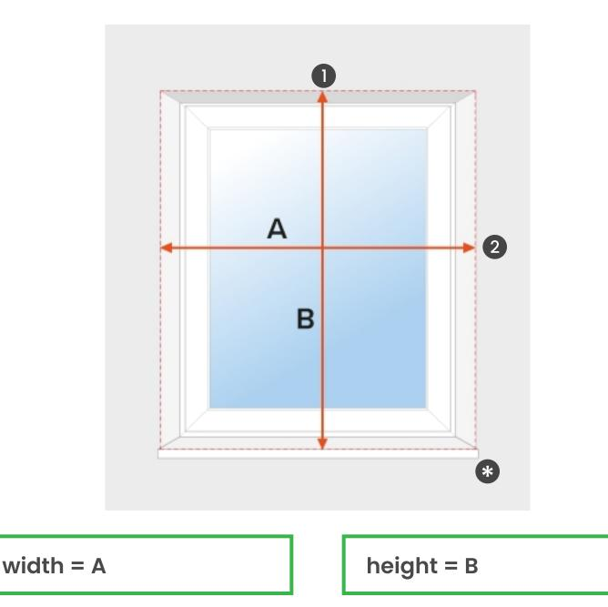
Measure the width and height of the window recess opening (outer edges of the recess).
