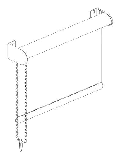
Installation to a wall, ceiling or window recess.
