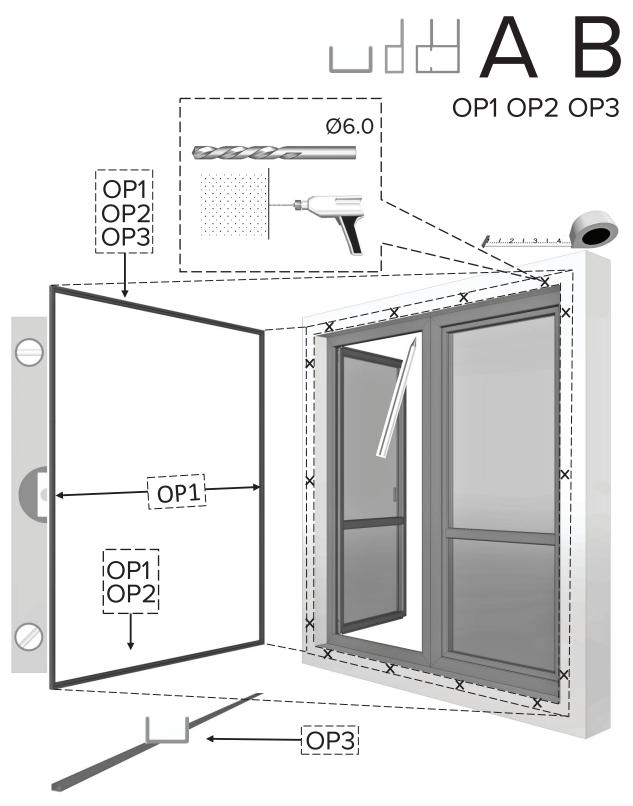
Once the slides have been prepared, try them on at the intended installation location and mark the limit points at which they are to be located, making it easier to move the required dimensions.
